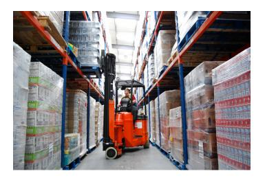
To enhance the aisle performance, High Reach Trucks are designed in a compact manner and this necessitates harder tyres to overcome stability issues resulting from the high centre of gravity. These smaller, harder tyres dictate that this type of truck is only suitable for inside work. More often than not a counterbalance truck is required to load vehicles from the warehouse.
