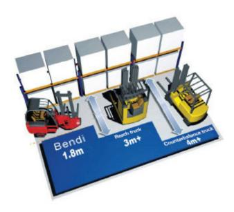
VNA (very narrow aisle) trucks are capable of working in much narrower aisles, approximately 1.7 - 2m, making the maximum use of storage space. This is the area in which UK forklift designer Freddy Brown was responsible for many developments prior to designing the original Bendi articulated truck.
